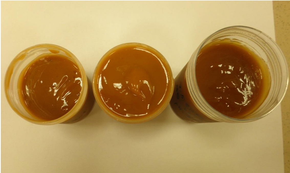
Figure 8. Visual image of effectiveness of incubation time of carbomer (from left to right: 0h, 1h, 20h)
