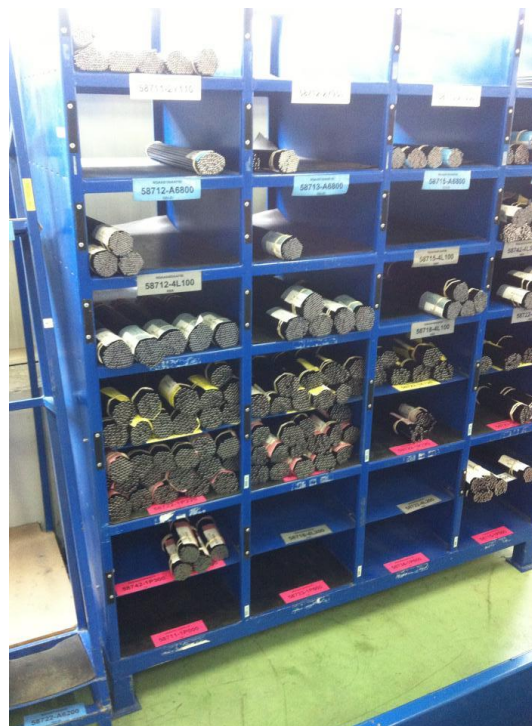
Figure 4-15 Supermarket at the cutting operation
