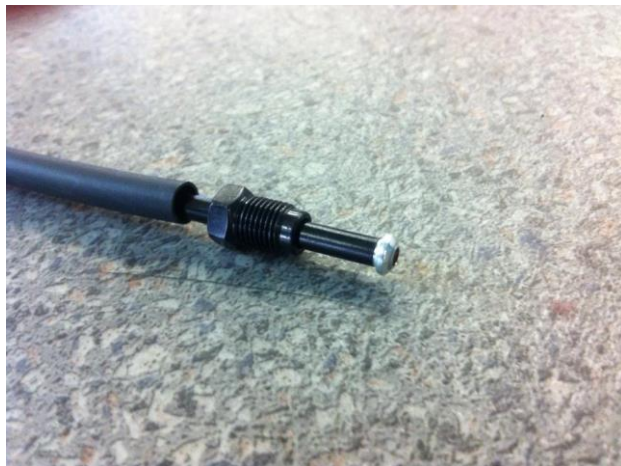
Figure 4-13 Pipe's end after pressing
