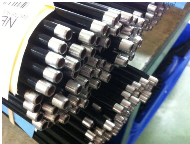
Figure 4-14 Smoothed surface after milling
