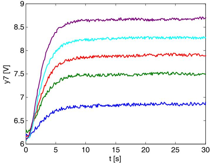
**Fig. 8.14** – Step responses of the system ( $u_2 - y_7$ ) for starting value  $u_2 = 5\text{ V}$
