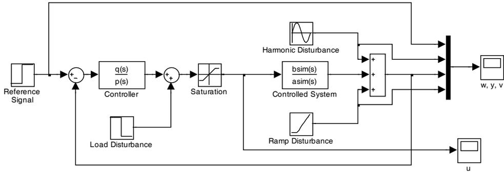
**Fig. 6.6** – SIMULINK scheme of 1DOF control system
