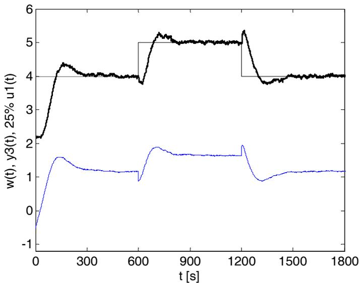
**Fig. 8.8** – Control of bulb temperature by regulator (8.13)
