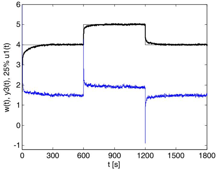
**Fig. 8.11** – Control of bulb temperature by regulator (8.19)
