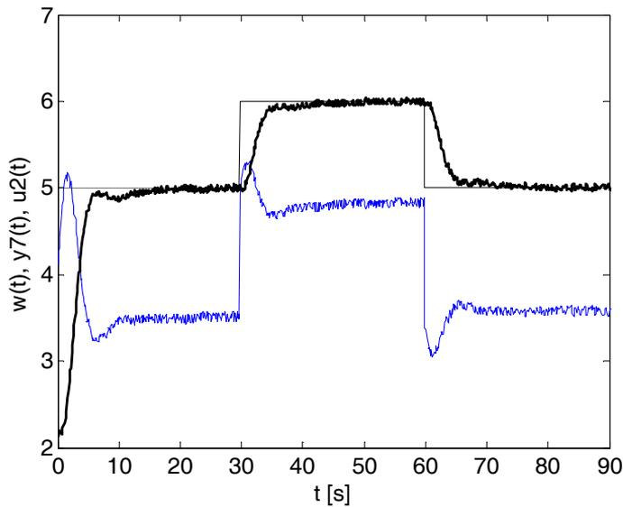
**Fig. 8.18** – Control of airflow speed by regulator (8.30)
