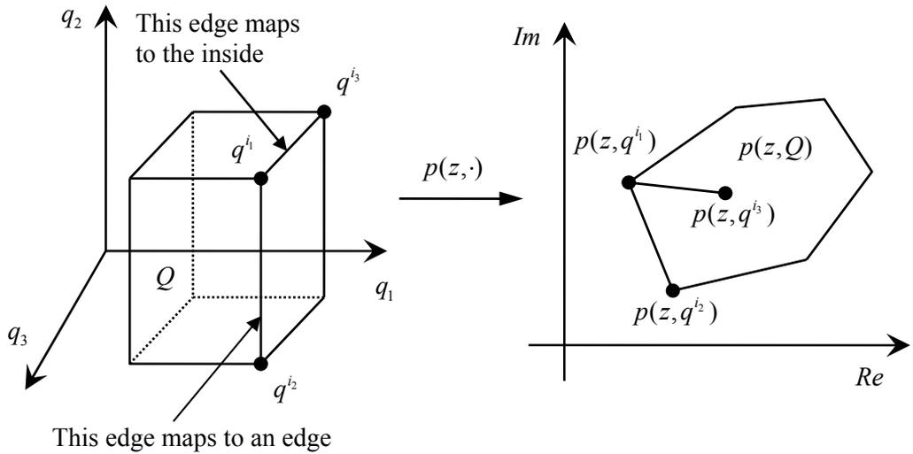
**Fig. 4.16** – Mapping an edge of  $Q$  into the interior of  $p(z, Q)$
