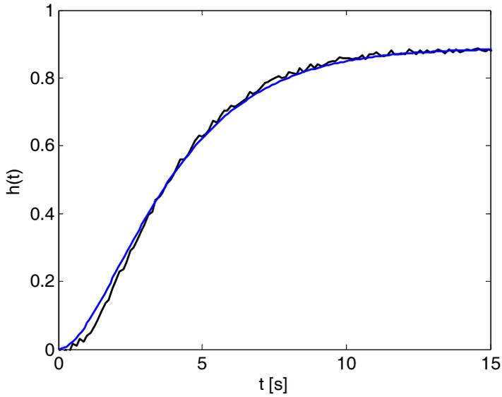
**Fig. 8.15** – Example of approximation by second order system with double time constant
