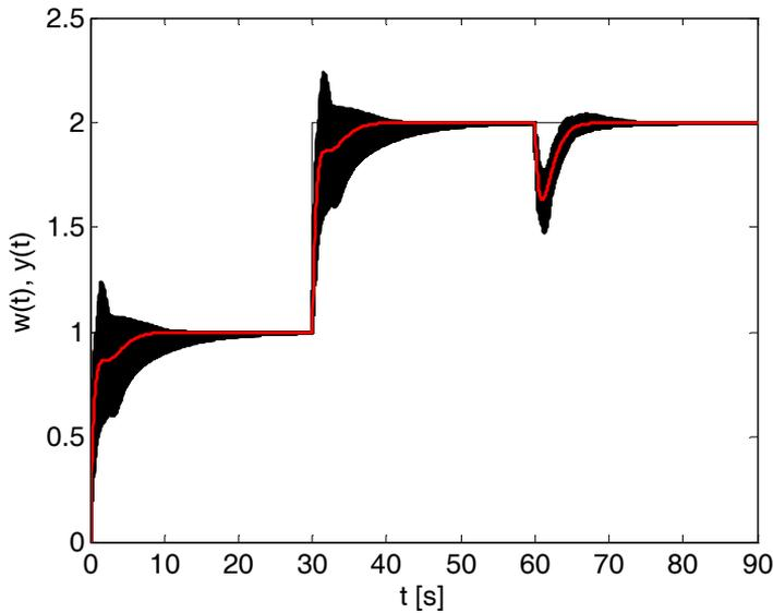
**Fig. 6.10** – Control of RSS of interval family (6.1) and nominal system (red curve) by controller (6.5)
