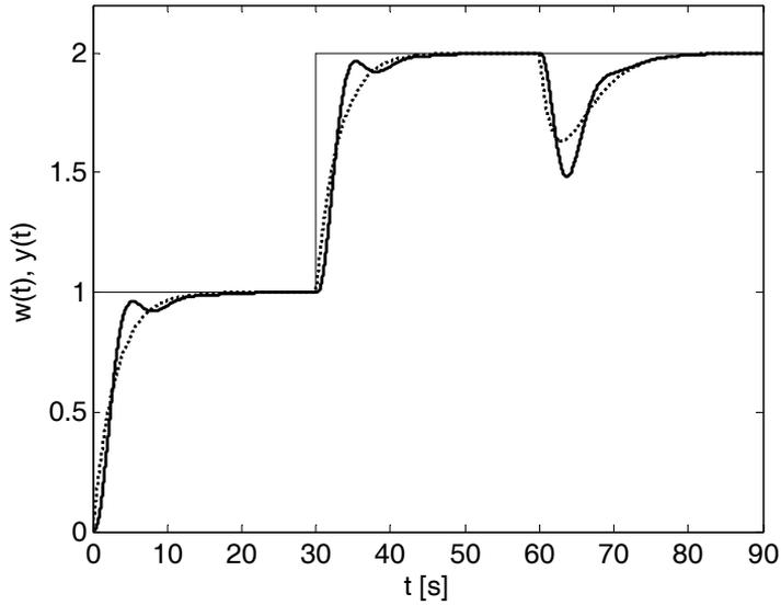
**Fig. 5.6** – The closed-loop control: PI regulator (5.76) for higher order system (5.72) (solid) and nominal one (5.74) (dotted)
