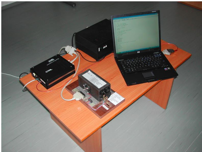
**Fig. 8.1** – Model of hot-air tunnel connected to PC via CTRL 51 unit
