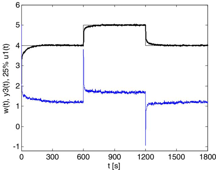
**Fig. 8.10** – Control of bulb temperature by regulator (8.18)
