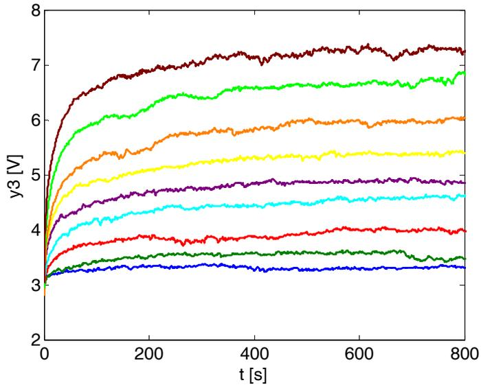
**Fig. 8.4** – Step responses of the system ( $u_1 - y_3$ ) for starting value  $u_1 = 0\text{ V}$
