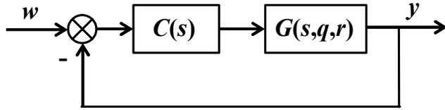
**Fig. 4.18** – Closed control loop with an interval plant
