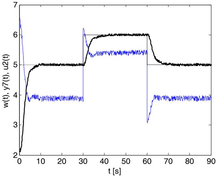
**Fig. 8.16** – Control of airflow speed by regulator (8.26)
