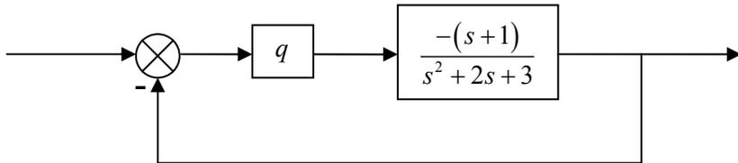
**Fig. 4.2** – The feedback system for example 4.2
