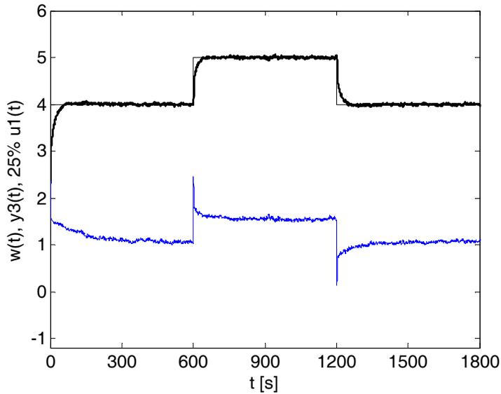
**Fig. 8.7** – Control of bulb temperature by regulator (8.10)
