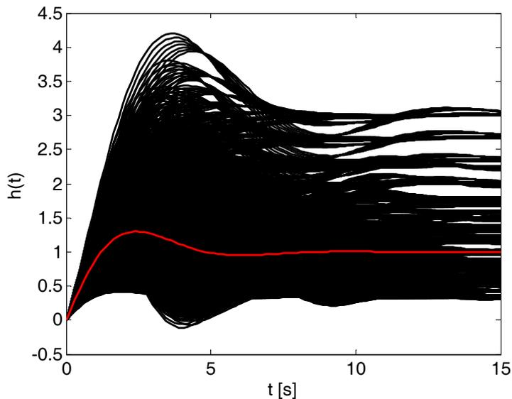
**Fig. 6.2** – Step responses of 2402 systems from interval family (6.1) – (the red curve represents the nominal plant)
