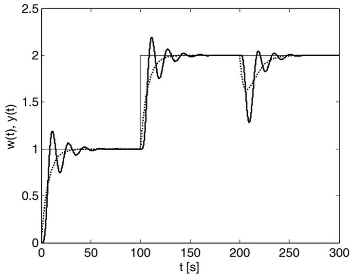
**Fig. 5.7** – The closed-loop control: PI regulator (5.77) for higher order system (5.73) (solid) and nominal one (5.75) (dotted)
