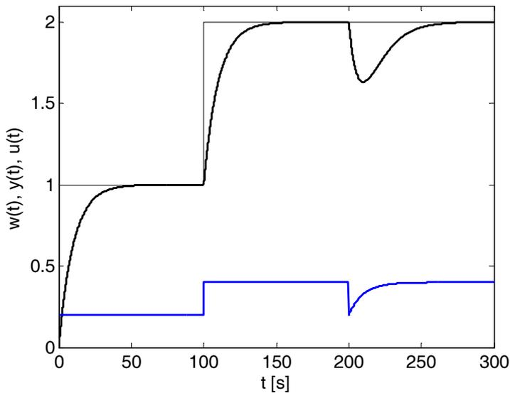
**Fig. 5.5** – Control behaviour of 1DOF system with plant (5.69) and controller (5.71) – control response (black), manipulated variable (blue)
