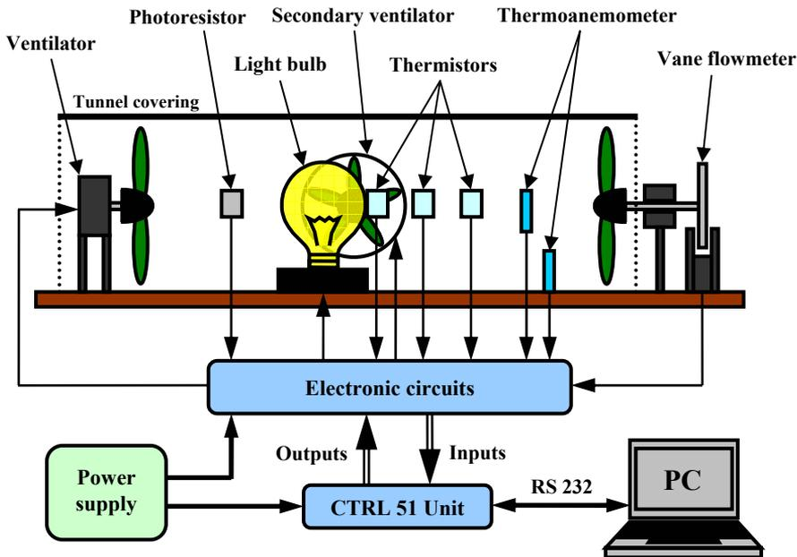
**Fig. 8.2** – Scheme of hot-air tunnel and whole control system
