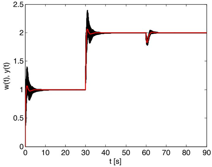
**Fig. 6.11** – Control of RSS of interval family (6.1) and nominal system (red curve) by controller (6.7) – 1DOF
