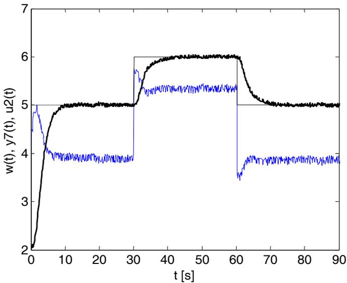
**Fig. 8.17** – Control of airflow speed by regulator (8.28)
