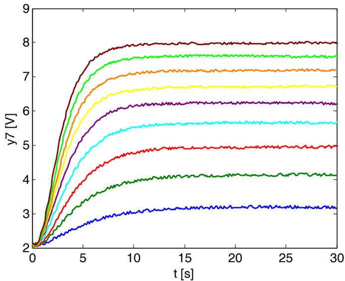
**Fig. 8.13** – Step responses of the system ( $u_2 - y_7$ ) for starting value  $u_2 = 1\text{V}$
