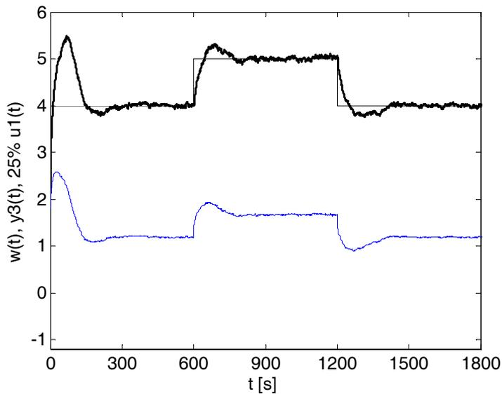
**Fig. 8.9** – Control of bulb temperature by regulator (8.15)
