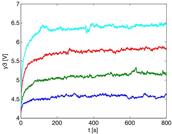
**Fig. 8.5** – Step responses of the system ( $u_1 - y_3$ ) for starting value  $u_1 = 5\text{ V}$
