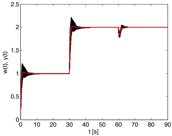
**Fig. 6.12** – Control of RSS of interval family (6.1) and nominal system (red curve) by controller (6.7), (6.8) – 2DOF
