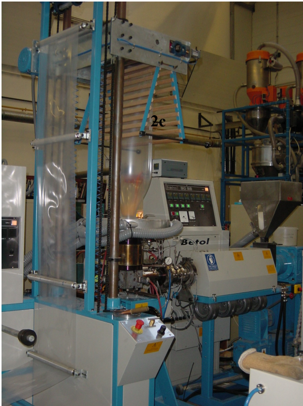
Fig. 33. Film blowing experimental set-up. 33a) General view of the experimental film blowing line; 33b) Closer view of the film blowing die; 33c) Used spiral mandrel.
