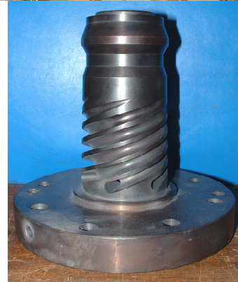
Fig. 33. Film blowing experimental set-up. 33a) General view of the experimental film blowing line; 33b) Closer view of the film blowing die; 33c) Used spiral mandrel.
