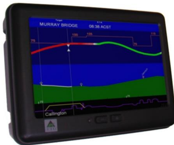
Obrázok 16: Fotografia zariadenia Energymiser (Trains to Cut Energy Use and Environmental Emissions, and Improve Overtime Running, with Energymiser – KiwiRail & TTG Transportation Technology Join Forces, 2013)
